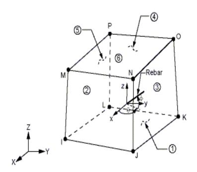
Figure 4: Element Geometry SOLID65 [17].
