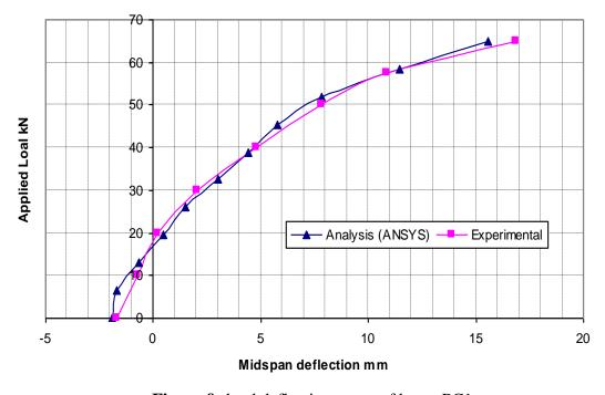
Figure 9: load deflection curve of beam PC1
