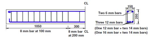
**Figure 8**: Reinforcement details of the concrete beam specimens (dimensions :mm)[1]
