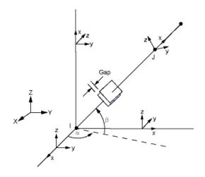
Figure 6:Element geometry CONTAC52[17].
