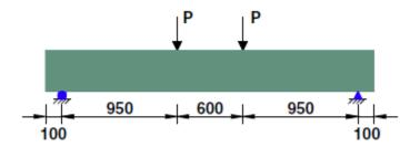
Figure 7: Loading configuration (dimension:mm)[1]
