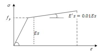
Figure3: Elastio-plastic stress-strain relationships for steel [18]
