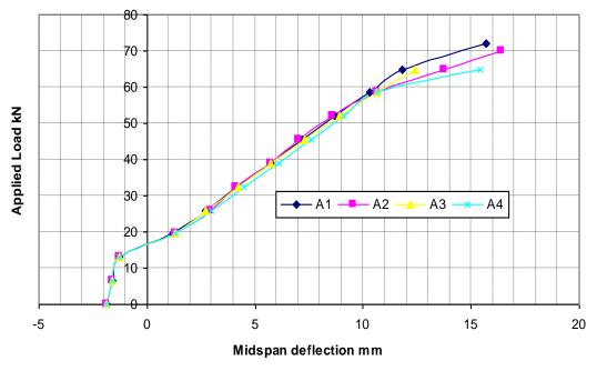
Figure 12: Effect of locations of prestressed CFRP plate
