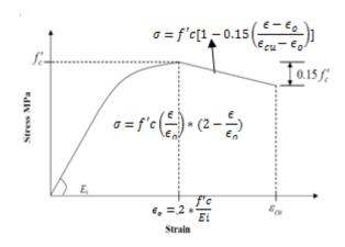
*Figure 1: Uniaxial stress-strain of concrete in compression*[16].
